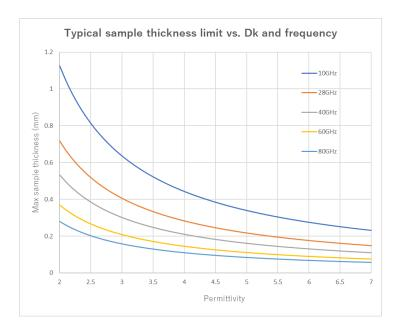
It is also necessary to cut the materials properly so that it fits well in the fixture. The following table provides the proper sample size for the resonators.
